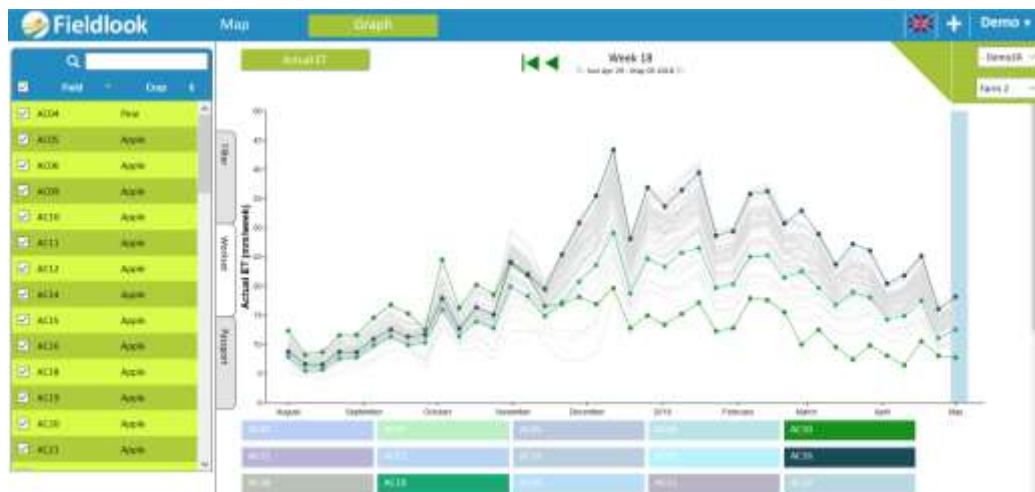
Figure 37. Example of field graphs showing actual evapotranspiration of 3 specific fields (coloured lines), compared to the other fields (light grey). These graphs provide crop statistics from the date of the crop emergence throughout the growing cycle. This allows the user to track crop status and identify fields that might need extra attention.
